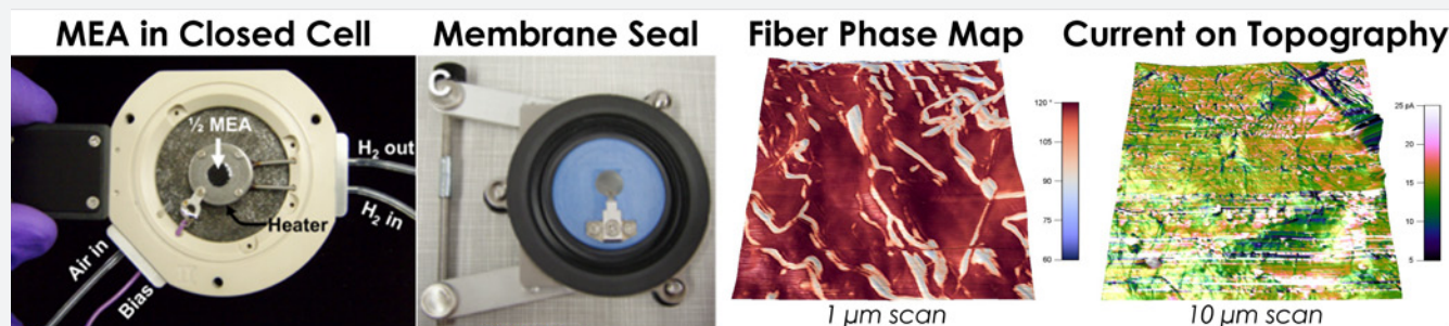
Figure 10. Phase and Conductive AFM mapping on a wetted anionic exchange membrane separator. (adapted from reference 8)
